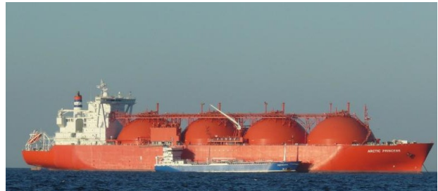
Fig. 4. LNG tanker "Arctic Princess" (Norway): L = 288 m, B = 49 m, T = 11.8 m, DWT = 74,400 t
