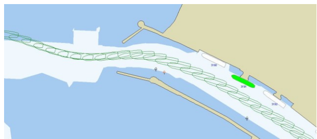
Fig. 5. LNG tanker sailing pass on departure in emergency situation (wind SW – 12 m/s, current out 1.2 kn, waves SW – 1.5 m) used four 50 T bollard pull tugs
