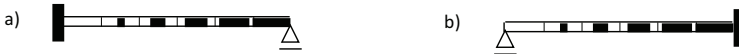
Fig. 6. The bands fixed on the one end and supported on hinge on the another end
