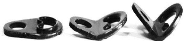
Fig.1. Illustrative photo of a seat belt anchor plate.
