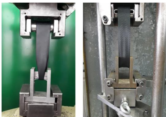
Fig. 5. Way of positioning a belt on the TST device in the pilot study
