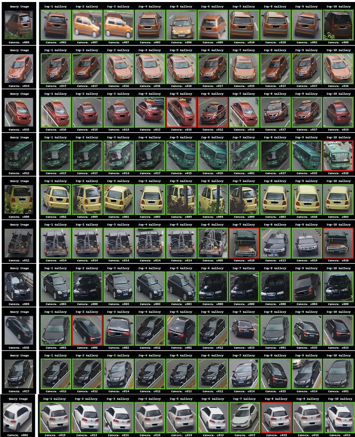
Figure 3. Qualitative results on VeRi dataset using BS based triplet embedding. Each row indicates query image and top-10 retrievals for this query image. Red border indicates an incorrect retrieval and Green indicates a correct retrieval. These demonstrate good embedding quality as the top retrievals include different views and cameras.
