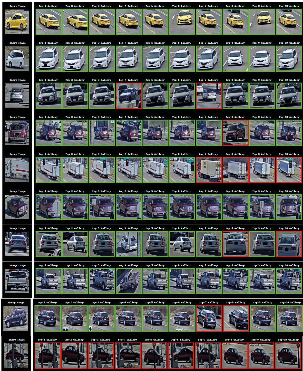
Figure 4. Qualitative results on CityFlow dataset. Red border indicates an incorrect retrieval and Green indicates a correct retrieval. Last row shows a failure case - due to a subtle shape mismatch on the trunk, and the presence of background-structure leading to poor embedding of the foreground object. In future work we would investigate incorporating segmentation information in training and retrievals.
