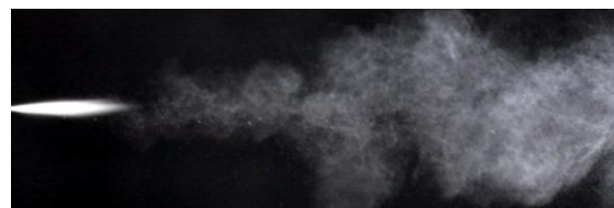
Fig. 1 The initial phase of the injection for ONM S-50 (see vapours from the previous injection)
