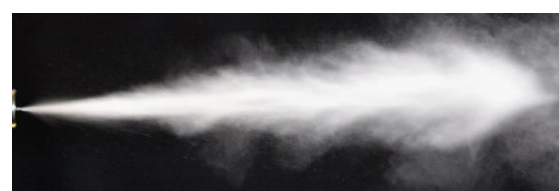
Fig. 3 Phase of full injection for ONM S-50 (see small vapour from the previous injection)
