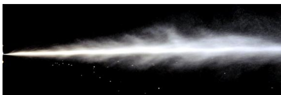
Fig. 7 Phase of full injection for EMKOR (see small vapour from the previous injection)
