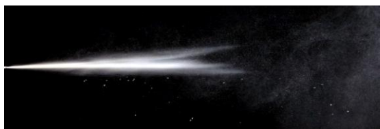
Fig. 6 Average advanced phase of injection for EMKOR
