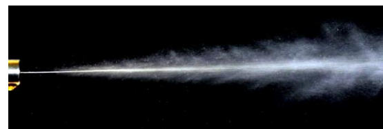
Fig. 11 Phase of full injection of OR100 (see small vapour from the previous injection)
