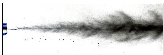
Fig. 8 Final phase of EMKOR fuel injection with visible jet fuel in the spray core and droplets everywhere
