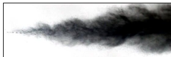
Fig. 4 Final phase of injection with visible droplets of ONM S-50 directly at the nozzle
