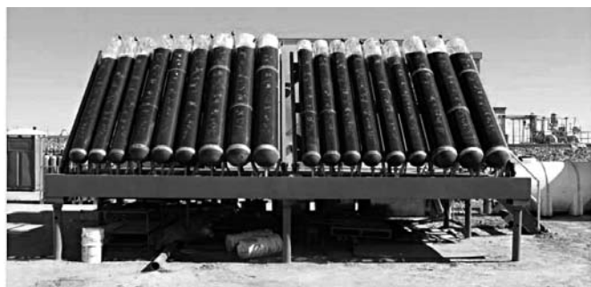
Fig. 8. Photobioreactor algae cultivation in Arizona (USA)
