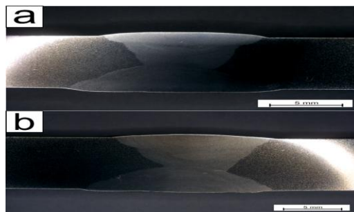
Fig. 7. Macrostructure of trial welded joints: a) state before annealing, b) annealed condition
