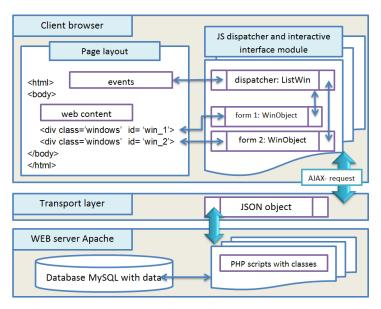
Fig. 3. Module components interaction scheme
