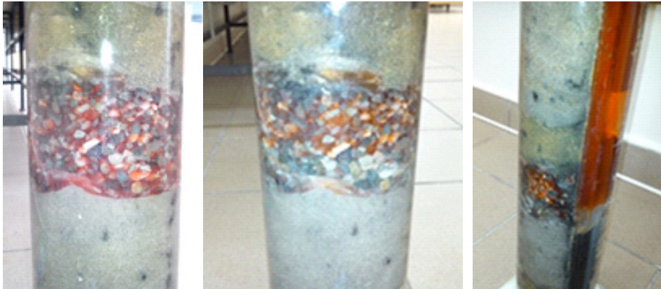
Fig. 4. LNAPL visible in the upper high permeable layer 1 day after its fourth addition (on the left) and 5 days after its fourth addition (in the middle and on the right [33])
