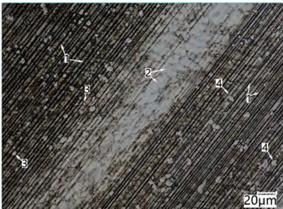
**Fig. 9. The surface of the padding weld 6070N worn in the presence of an abrasive slurry: 1 – ploughing, 2 – chromium carbides, 3 – vanadium carbides, 4 – niobium carbides**
