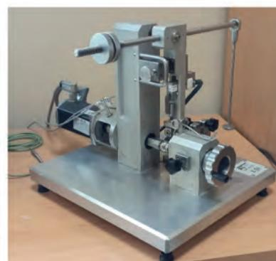
**Fig. 4. Scheme and general view of the T-20 stand for testing the abrasive wear using the ball-cratering method: 1 – sample, 2 – ball (counter-sample), 3 – sample holder arm, 4 – load, 5 – counterweight, 6 – pivot**
