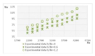
Fig. 3. Nusselt number as a function of air Reynolds number evaluated from experimental results of heat exchanger which is placed in underpart of air-handling unit
