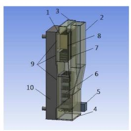
Fig. 1. Combined shock-foam-type air-handling unit with a block of thermoelectric modules design: 1 - air-conditioner cabinet; 2 - inlet opening; 3 - out let opening;
