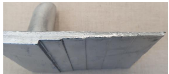
Fig. 2. AlSi6Cu4 step-casting from the metal mold
