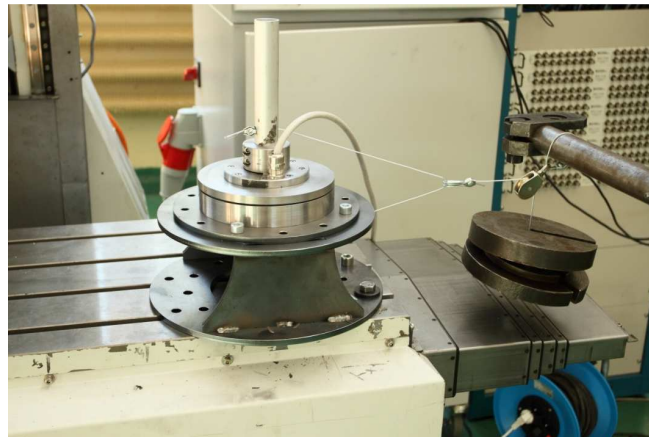
Fig. 8. The experimental stand for calibration of the joystick measurement system
