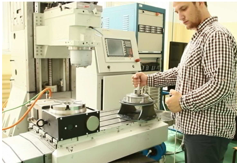
Fig. 10 Designed joystick connected to CNC machine during functional test performed by operator
