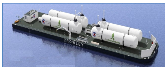
Fig. 4 Inland waterways LNG barge designed by Jensen Maritime
