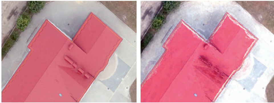
Fig. 2. Fragments of a building's image on a traditional orthophotomap (left) and on the orthophotomap designed using the proposed method (right)
