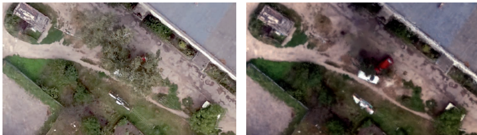
Fig. 2. Fragments of a building's image on a traditional orthophotomap (left) and on the orthophotomap designed using the proposed method (right)
