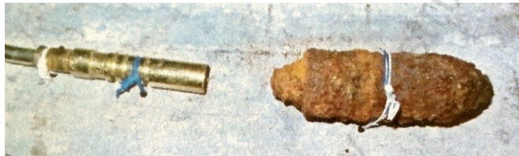
Fig. 6. Field test of the projectile for the presence of explosives
