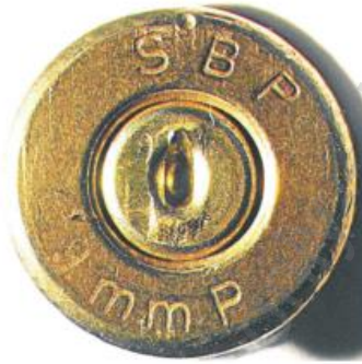
Fig. 1. Characteristic marks left by the ejector, extractor and firing pin on a cartridge case fired from GLOCK pistol. Ammunition producer stamp and calibre are visible
