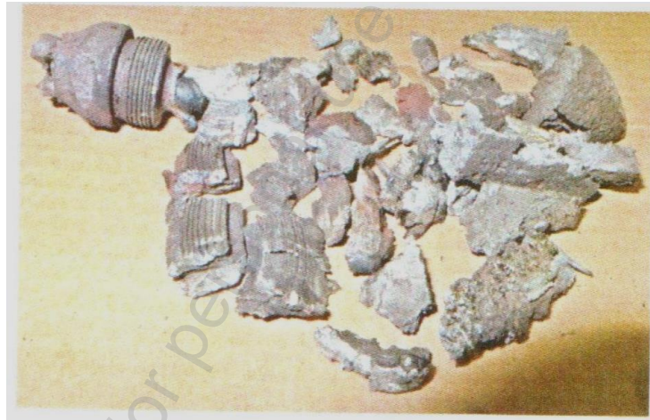
Fig. 7. Fragments generated as the result of projectile detonation
