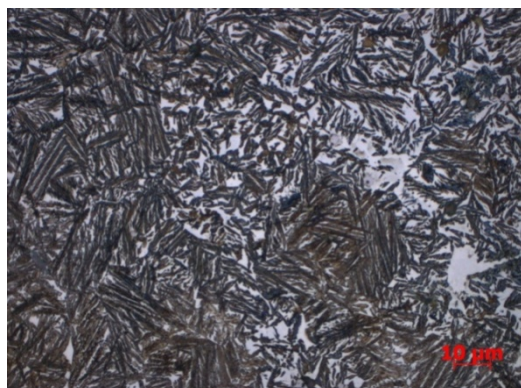
Fig. 4. Microstructure of ADI from C1 cycle. Etched with Beraha reagent - Martensite, 1000x. Pre-eutectoid ferrite, lower bainite, austenite
