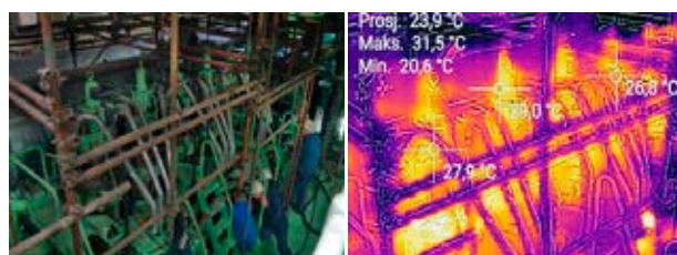
Figure 8. Visible light image (left) and thermal image (right) of the upper part of a ship's main propulsion engine
