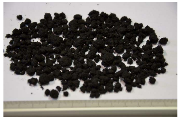
Fig. 2. Pellets in moulding sand
