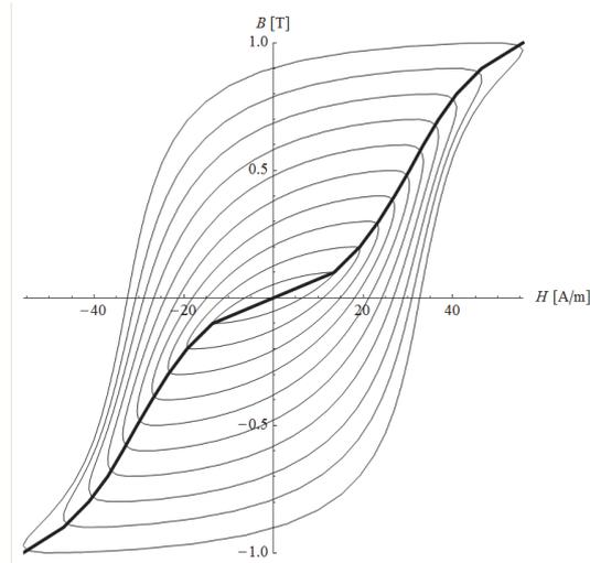
Fig. 6. Hysteresis loop family obtained from measurements for  $f=400$  Hz, BNO 6.5% Si; also vertex magnetization curve is depicted
