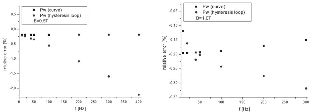
Fig. 8. Relative error for eddy current power loss calculated according to the algorithm related to the classic loss,  $B=0,5$  T and  $B=1.0$  T, BNO 6.5% Si (black squares – calculations with vertex curve, red dots – calculations with hysteresis loop family)
