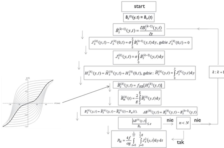
Fig. 2. Block diagram of the algorithm
