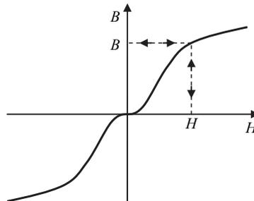
Fig. 3. Conversion  $H \rightarrow B$  and  $B \rightarrow H$  by vertex curve
