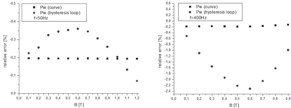
Fig. 7. Relative error for eddy current power loss calculated according to the algorithm related to the classic loss,  $f=50$  Hz and  $f=400$  Hz, BNO 6.5% Si (black squares – calculations with vertex curve, red dots – calculations with hysteresis loop family)
