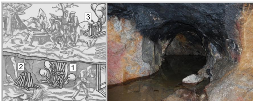
Fig. 3. Principle of fire-setting (according Agricola, 1556): (1) kindled logs, (2) heap of dried logs, (3) fumes ventilation; photo illustrates an example of the rest of soot on the roof of gallery ( photo: Lednická )
