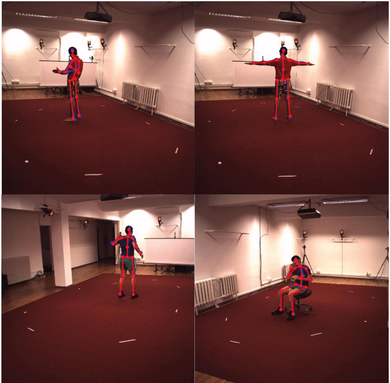
Figure 10. An illustration of 2D human pose estimation on the Human 3.6M dataset (Protocol #1 - Subject 9, Subject 11). The blue skeleton are the ground truth skeleton, the red skeleton are the estimated skeleton.
