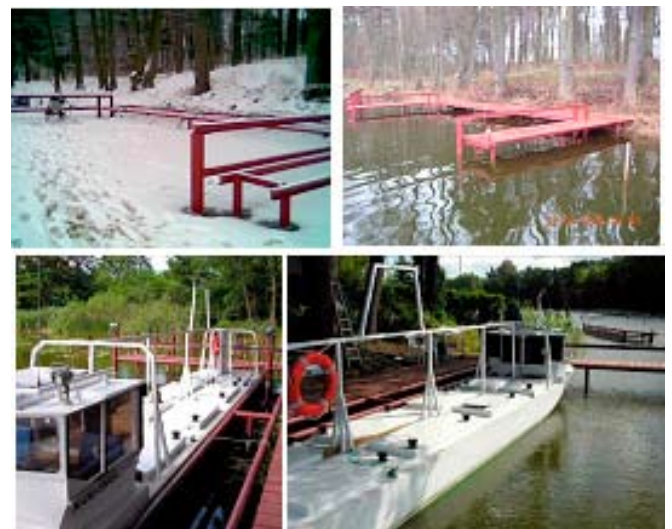
Figure 5. Experimental stand under construction and the man manned scale model of a ferry during the tests in the research area of Ship Handling Research and Training Center in Ilawa-Kamionka.
