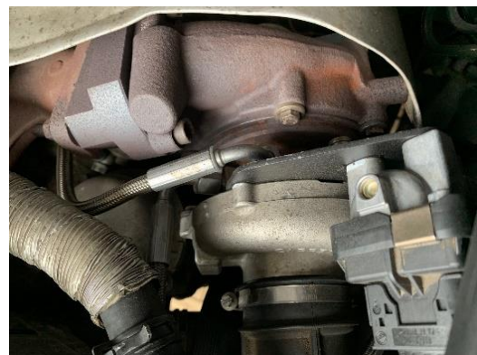
Fig. 6 Picture of new VNT turbocharger
