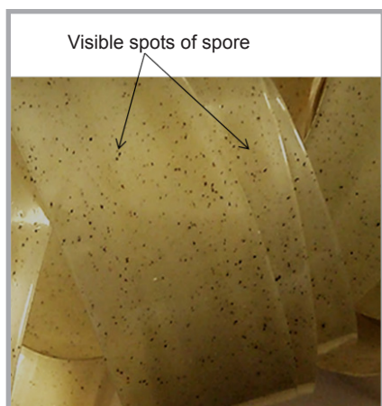
Figure 3. Photograph of PET film embedded with spores showing visible spots of spores on the film surface (indicated by arrows).
