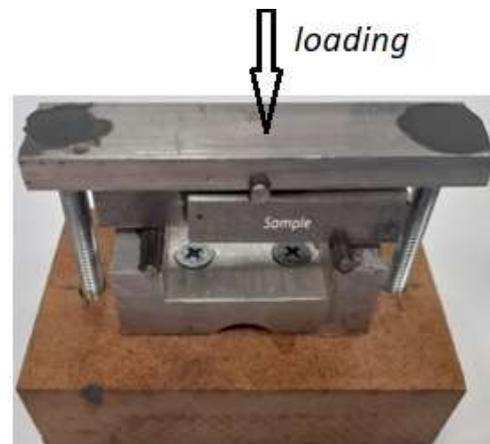
Fig. 4. The sample mounted in the device for testing the static strength by bending
