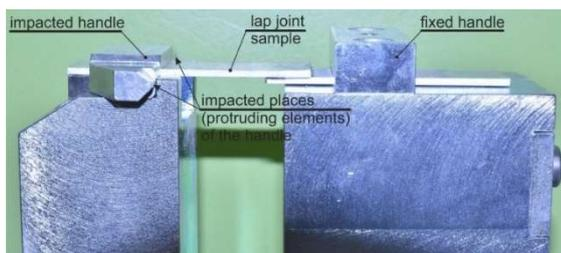
Fig. 2. Method of fixing lap specimens in impact tests
