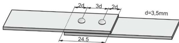
Fig. 1. The spacing of rivets in the lap sample, loaded by tension
