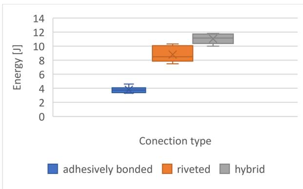
Fig. 8. Comparison of the failure energy of different types of joints of lap specimens loaded by bending
