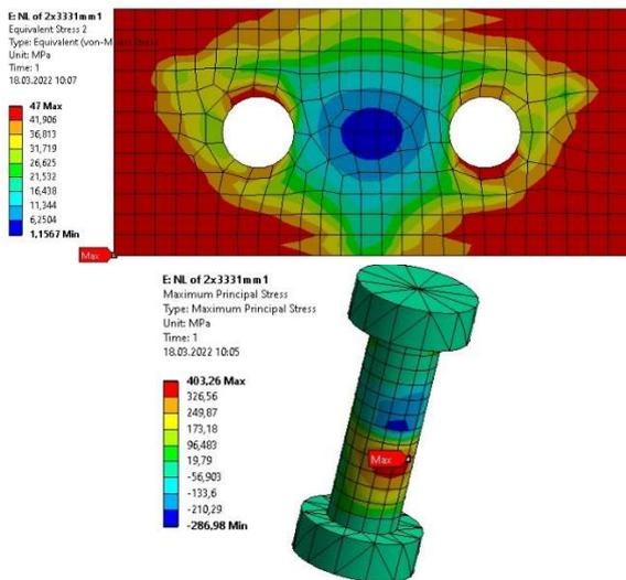
Fig. 17. Mises stress distribution in the adhesive layer and in the rivet body of a hybrid joint loaded by bending with a force of 6662 N (nonlinear properties of the adhesive and aluminum alloy)
