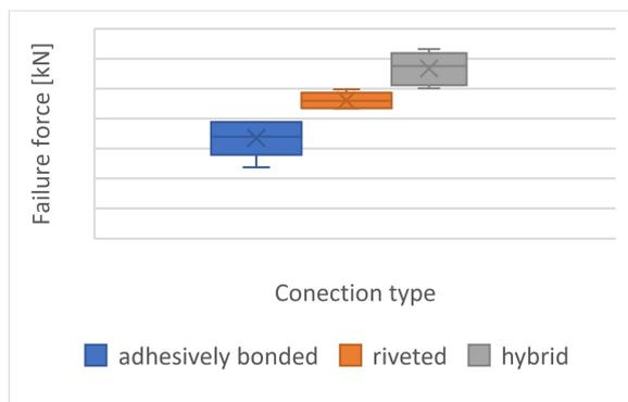
Fig. 5. Comparison of the resistance of different types of joints of lap specimens loaded by tension (X - median, mustache - maximum and minimum value, box - range 50% of the results (difference between the third and first quartile))
