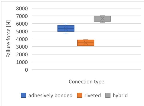
Fig. 7. Comparison of the resistance of different types of joints of lap specimens loaded in shear by bending
