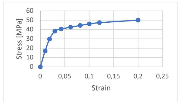
Fig. 14. The curve  $\sigma = \sigma(\epsilon)$  of Loctite EA 9664 adhesive
