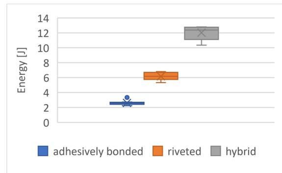
Fig. 6. Comparison of the failure energy of different types of tension lap joints
