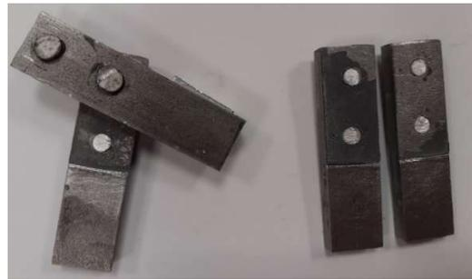
Fig. 9. Two methods of destroying hybrid lap joints of bended samples
