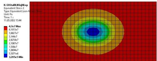
Fig. 15. Mises stress distribution in the adhesive layer of the joint loaded by bending with a force of 5347 N (nonlinear properties of the adhesive)
