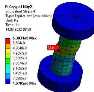
Fig. 16. Mises stress distribution in the shaft of a mechanical connector of a riveted joint loaded by bending with a force of 3504 N (nonlinear properties of aluminum alloy)
