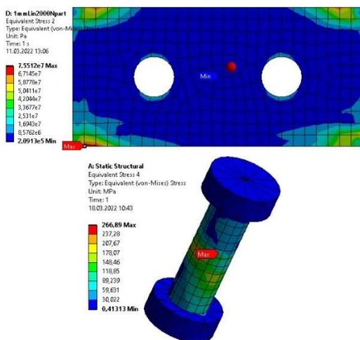
Fig. 13. Mises stress distribution in the adhesive layer and in the rivet body of a hybrid joint loaded by bending with a force of 2000 N
