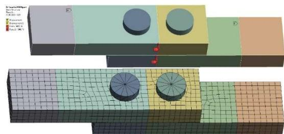
Fig. 10. The way of loading the hybrid connection and the mesh of elements
