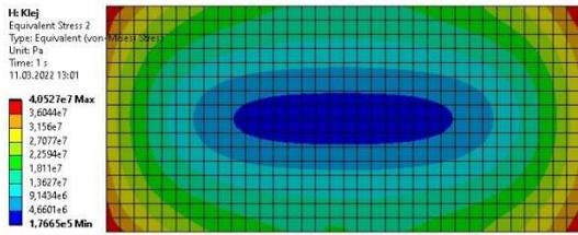
Fig. 11. Mises stress distribution in the adhesive layer of the joint loaded by bending with a force of 2000 N
