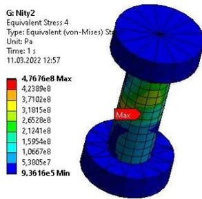
Fig. 12. Mises stress distribution in the shaft of the mechanical connector of a riveted joint, loaded by bending with a force of 2000 N
