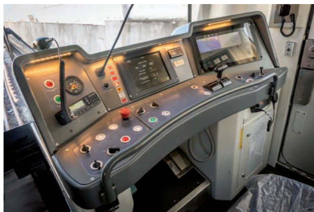
Fig. 22. The control panel on the Varsovia train [photo: Škoda]
