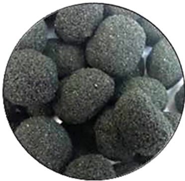
Fig. 11. Precursors – Furan molding mixture (regular shape and size)
