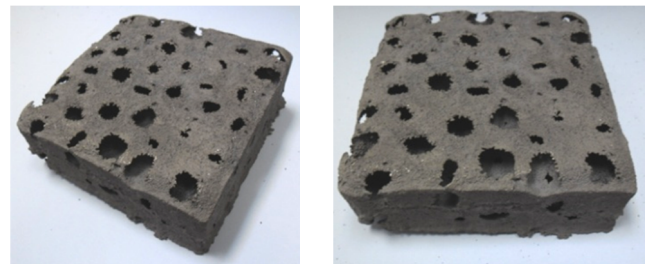
Fig. 8. Casting (CuSn10) – type I
