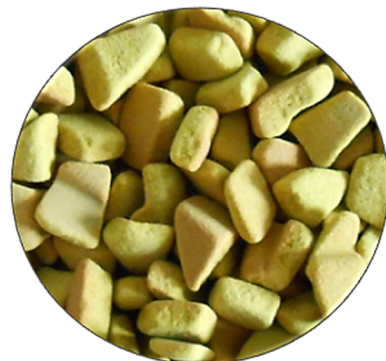
Fig. 10. Precursors – Croning process (irregular shape and size)
