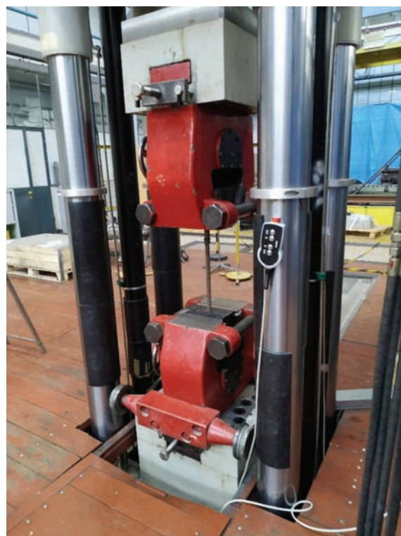
Fig. 4. Test stand – universal testing machine [photo: M. Ostromęcka]
