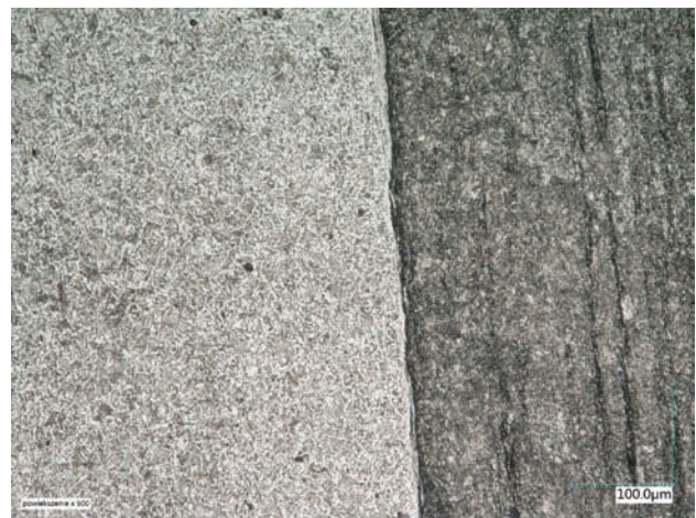
Fig. 6. Microstructure of the dissimilar welded joint between B500B and 1.4021 steel; on the left the microstructure of the B500B reinforcing steel, on the right the structure of the martensitic steel with distinct fibrousness; microstructure in the initial state before tension [photo: M. Ostromęcka]
