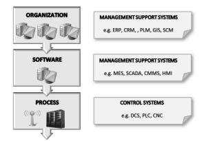
Fig. 1. Structure of IT tools supporting individual process layers (Kosicka & Mazurkiewicz, 2015)
