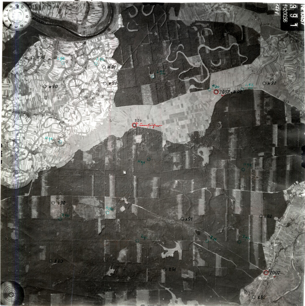
Figure 3. Archival aerial photograph of the area around Nowe Brzesko, probably from 1944, at the approximate scale of 1:46,000; Rb30/20 camera, focal length: 200.56 mm (National Archives and Records Administration, reference no. TU GX 895A SK, photo no.391)
