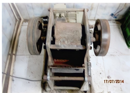
Fig. 1. The device used for crushing and grinding the pumice
