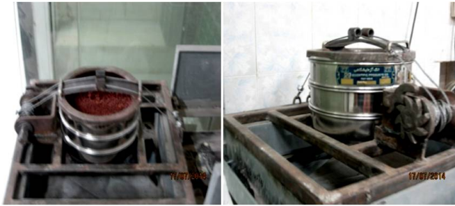
Fig. 2. Placement of the sieves on top of each other
