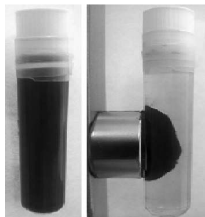
Fig. 1. Magnetic separation of superparamagnetic nanoparticles dispersed in liquid media. The separation-redispersion cycles can be repeated indefinitely. Originally suspended (left) were attracted to the side of a permanent magnet (right) after 5 min.
