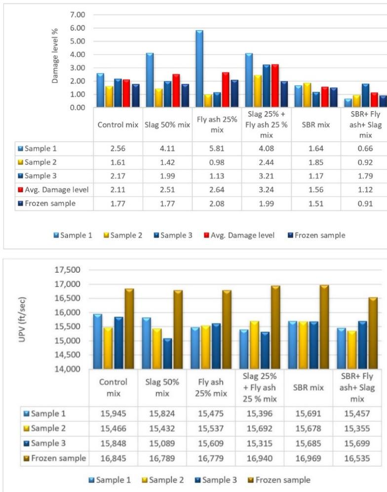
**Fig. 4.** Damage levels and average UPV values
