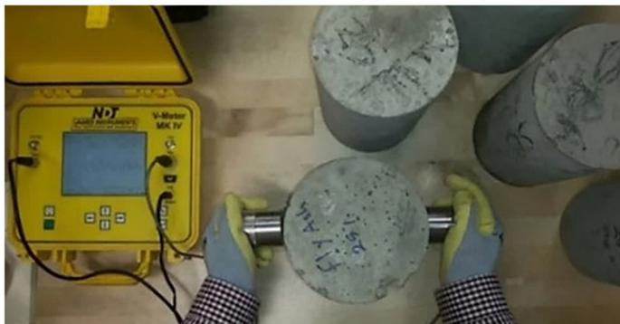
**Fig. 1.** Concrete samples and UPV test
