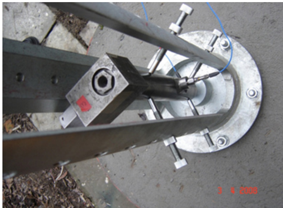
Figure 3. A ballistic test rocket motor installed on a vertical ballistic test stand – view from the engine nozzle side
