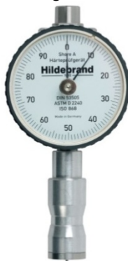
Fig.6. The device for measuring hardness by Shore's method [9]
