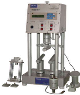
Fig. 5. The workstation for bending strength testing [8]
