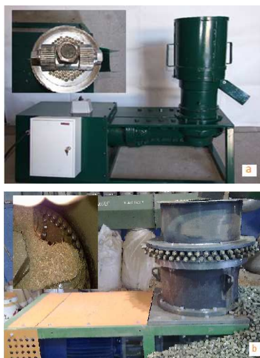
Fig. 1. Pictures of the used pelleting machines: a) with flat matrix, b) with ring matrix
