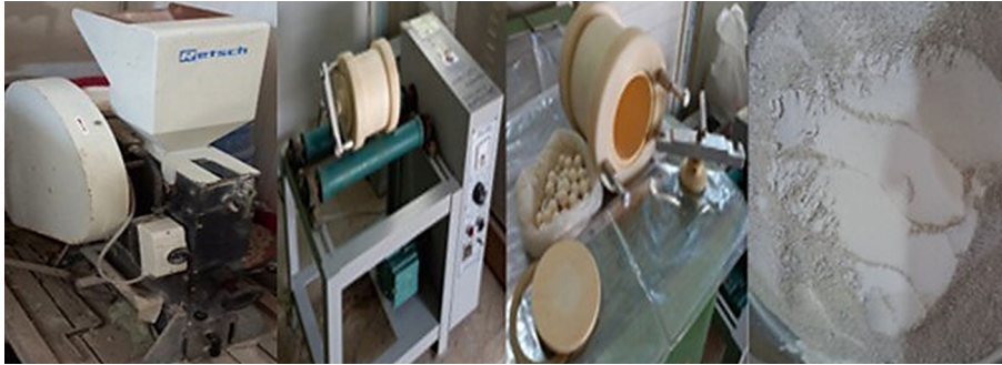
Fig. 2. Crusher and ceramic ball mill device
