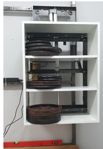
Fig. 10. Schematic diagram of the upper cabinet mechanism, side view of the prototype mechanism with the cabinet, cabinet with the mechanism during tests with asymmetric loading.
