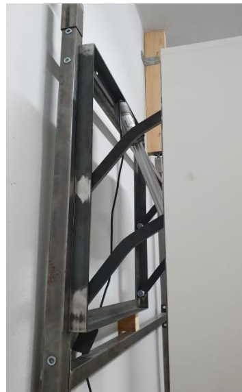
Fig. 10. Schematic diagram of the upper cabinet mechanism, side view of the prototype mechanism with the cabinet, cabinet with the mechanism during tests with asymmetric loading.
