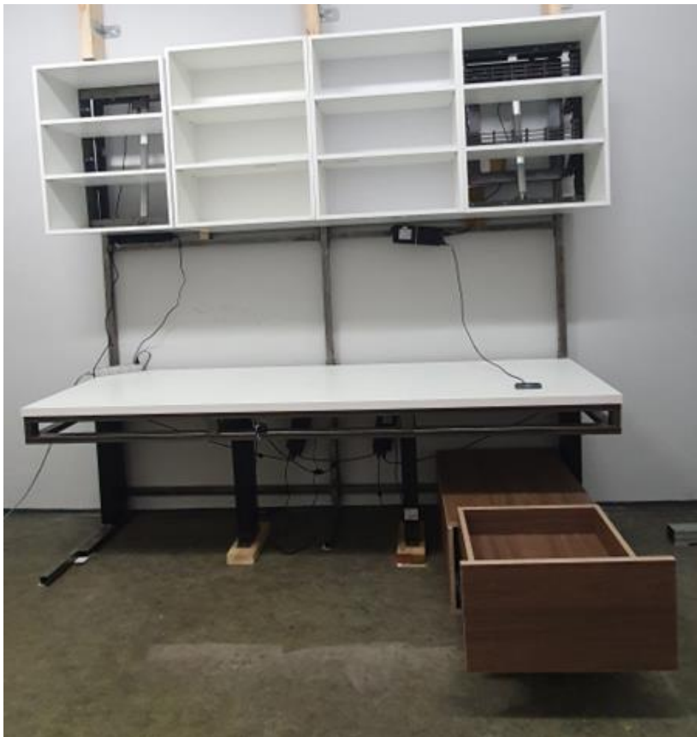
Fig. 13. Integrated structures: load-bearing frame, lifting and lowering systems for two upper cabinets (above the countertop), lifting and lowering system for the countertop, and drawer extension and lifting system under the worktop.
