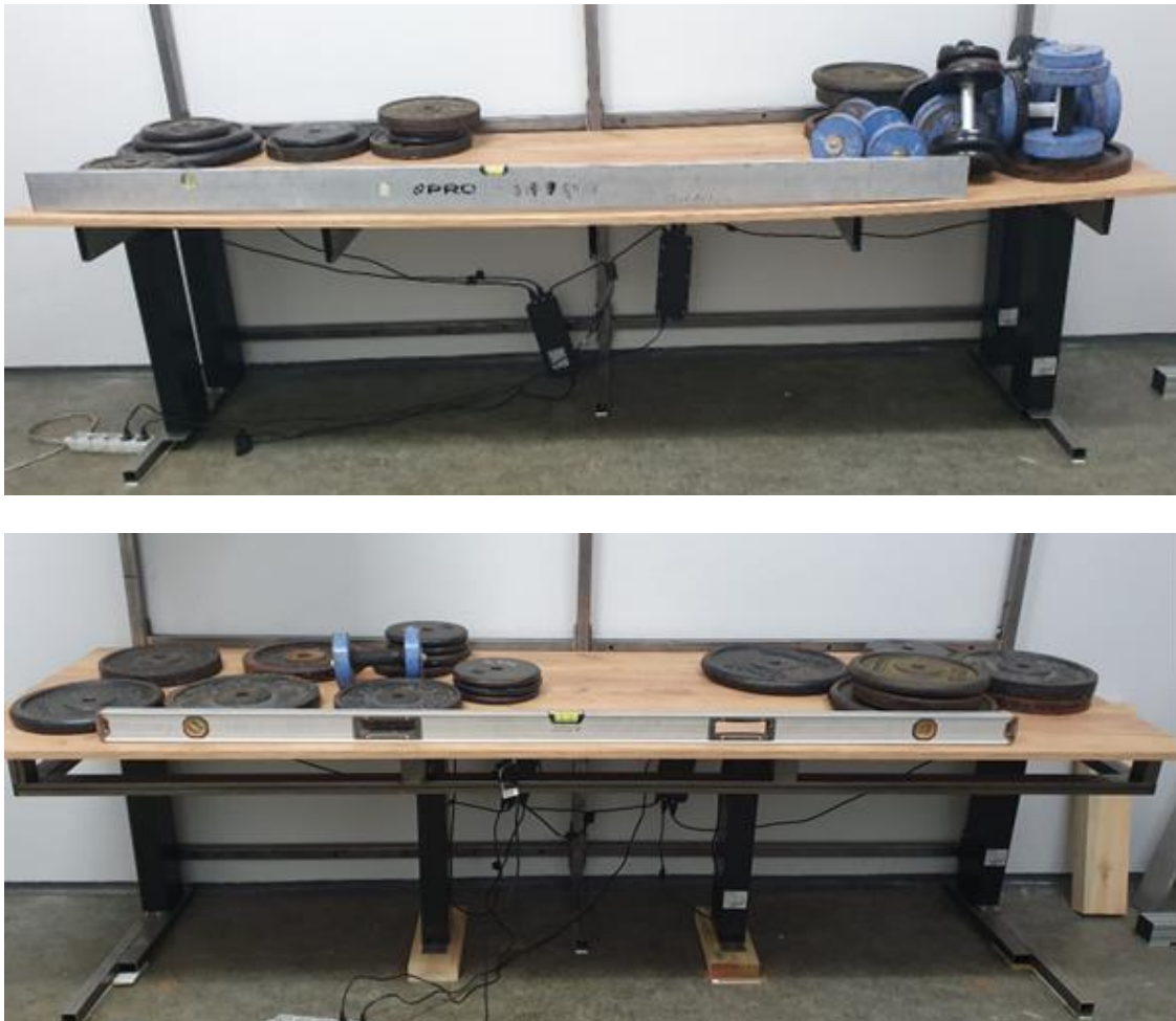
Fig. 11. Countertop lifting system during load testing. At the top, the first version of the system without a frame for attaching the countertop, and at the bottom, the second version of the system - the final version, with a sturdy frame for attaching the countertop element.
