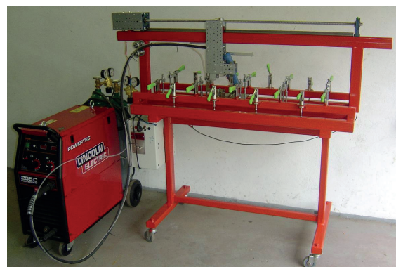
Fig. 1. Apparatus for welding with micro-jet cooling
