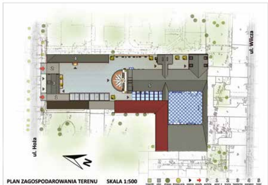
Fig. 7. Land development plan. Designed division of the external space, along with adjacent buildings. 1 – Entrance to the underground garage, 2 – additional function buildings, including a cafe, 3 – main entrance gate, 4 – office rooms for rent, 5 – main building with a hotel function, along with the adjacent atrium and newly designed buildings; source: author
