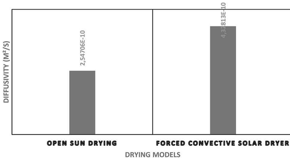
Figure 4. The value of the effective diffusivity of drying bay leaves in the CSD and OSD drying systems
