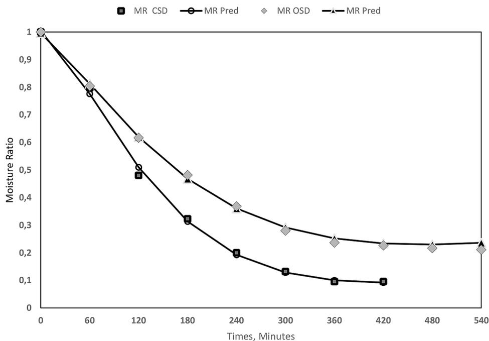
**Figure 3.** Modeling the drying of bay leaves using the Midilli equation on the OSD and CSD drying system
