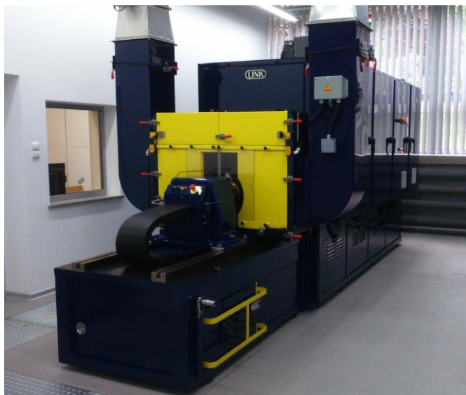
Picture 1. The LINK M3000 Inertia Brake Dynamometer.
