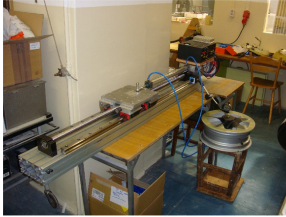
Fig. 3. The fatigue stand for the rotor of the MOSUPS propulsion system
