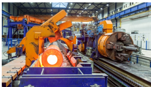
Rys. 7. Rura wsadowa do kucia rur grubościennych na kowarce SMX 800/18 MN w Vitkovicie – Czechy [6] Fig. 7. Initial tube for forming thick-walled tubes on SMX800/18MN forging machine in Vitkovice in Czechia [6]
