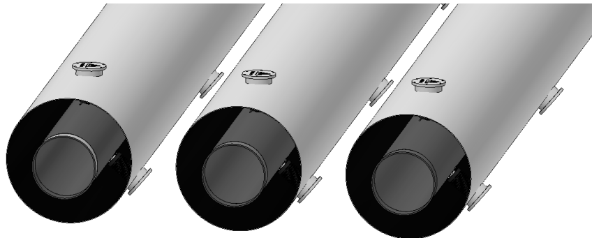
Fig. 2. Single-pole high-currents busduct [11]
