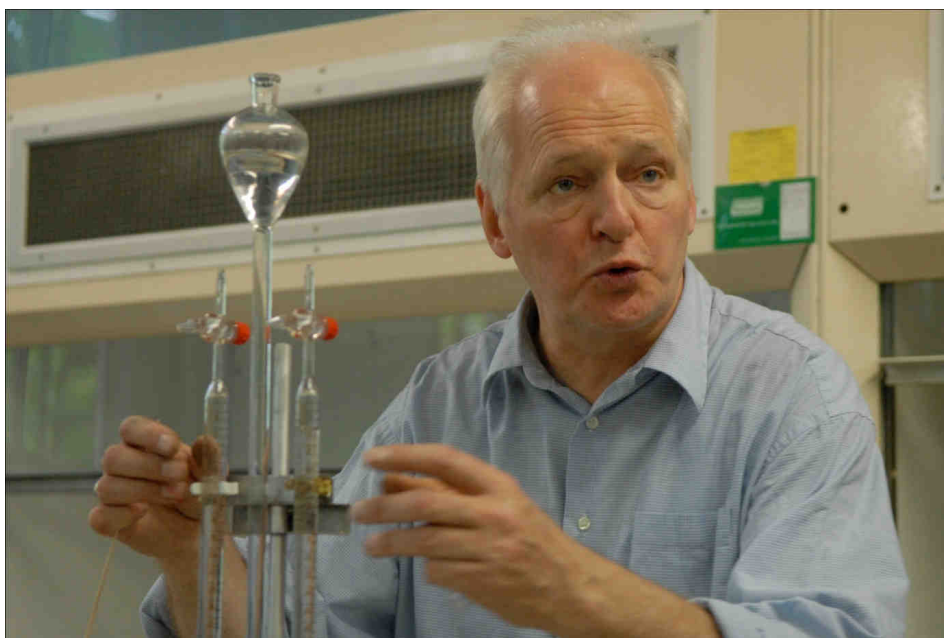
Fig. 7. The Hofmann Voltmeter (1866) shows one of the most significant experiments of the 19th century - this is the decomposition of water (which for centuries had been considered to be an element) into hydrogen and oxygen
