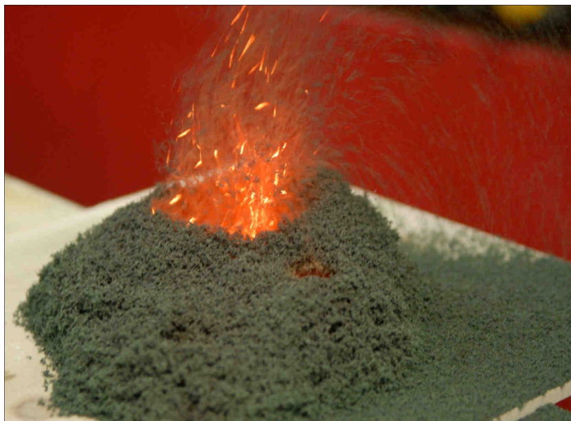
Fig. 5. The ammonium dichromate volcano is spectacular for its colour change and also the huge increase in volume of solid
