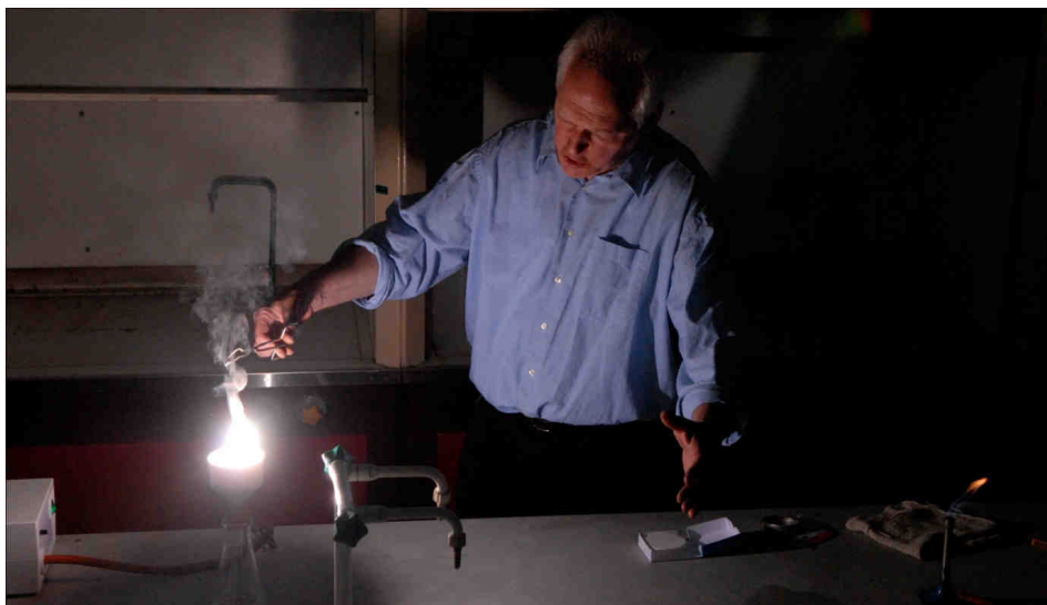
Fig. 6. The photolytic decomposition of silver bromide illustrates the reaction which underlies “traditional” photography. In this reaction we burn magnesium ribbon over a metal object which covers freshly precipitated silver bromide - the result is an impressive photogram of the metal object
