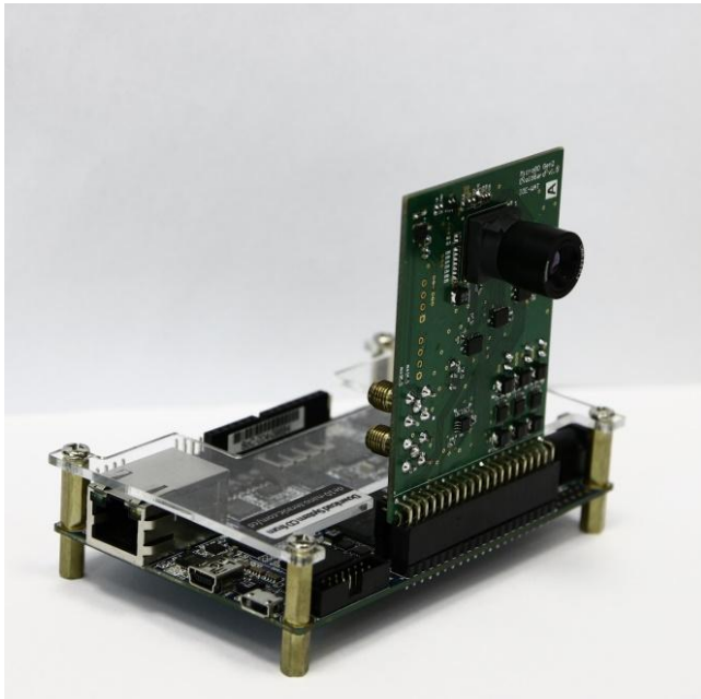
Fig. 2. The view of the Acquisition assembly consisting of interface PCB and DE10-Nano board
