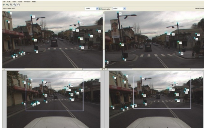
Fig. 9. Measured 18 points on the measurable images selected from the road test.
