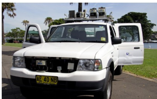
Fig. 5. Multi-sensors mounted on the vehicle
