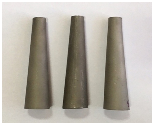
Fig. 5. Test specimens made of Inconel 713C
