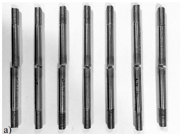
Fig. 6. Determination of the DRT: a) Samples for testing, b) view of the Gleeble 3500 simulator chamber with a specimen fixed in it
